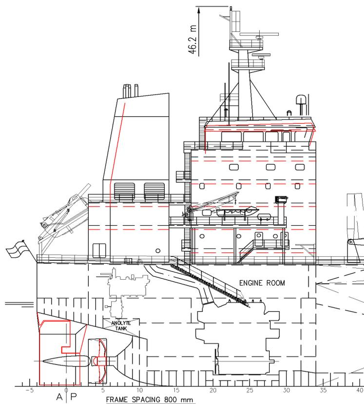
Aft body with modifications, including speed nozzle, spade rudder, Costa bulb, increased funnel and elevated accommodation block.
